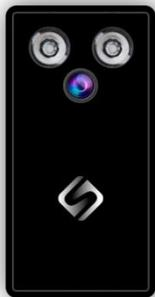
To make the search and detection of hidden video cameras more simple in the kit of "ARCANE" provided a special identifier of hidden video cameras lenses. Direct it to the suspected location of the camera, the surface of the wall or ceiling (detected by the ARCANE device), turn on the backlight - and by seeing a bright dot indicating the location of the lens, detecting the "hidden" camera behind it.
