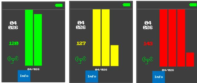
The screen will display graphs of received signal level, the number and color of which varies, depending on the signal level when approaching or moving away from the signal source (video camera).
