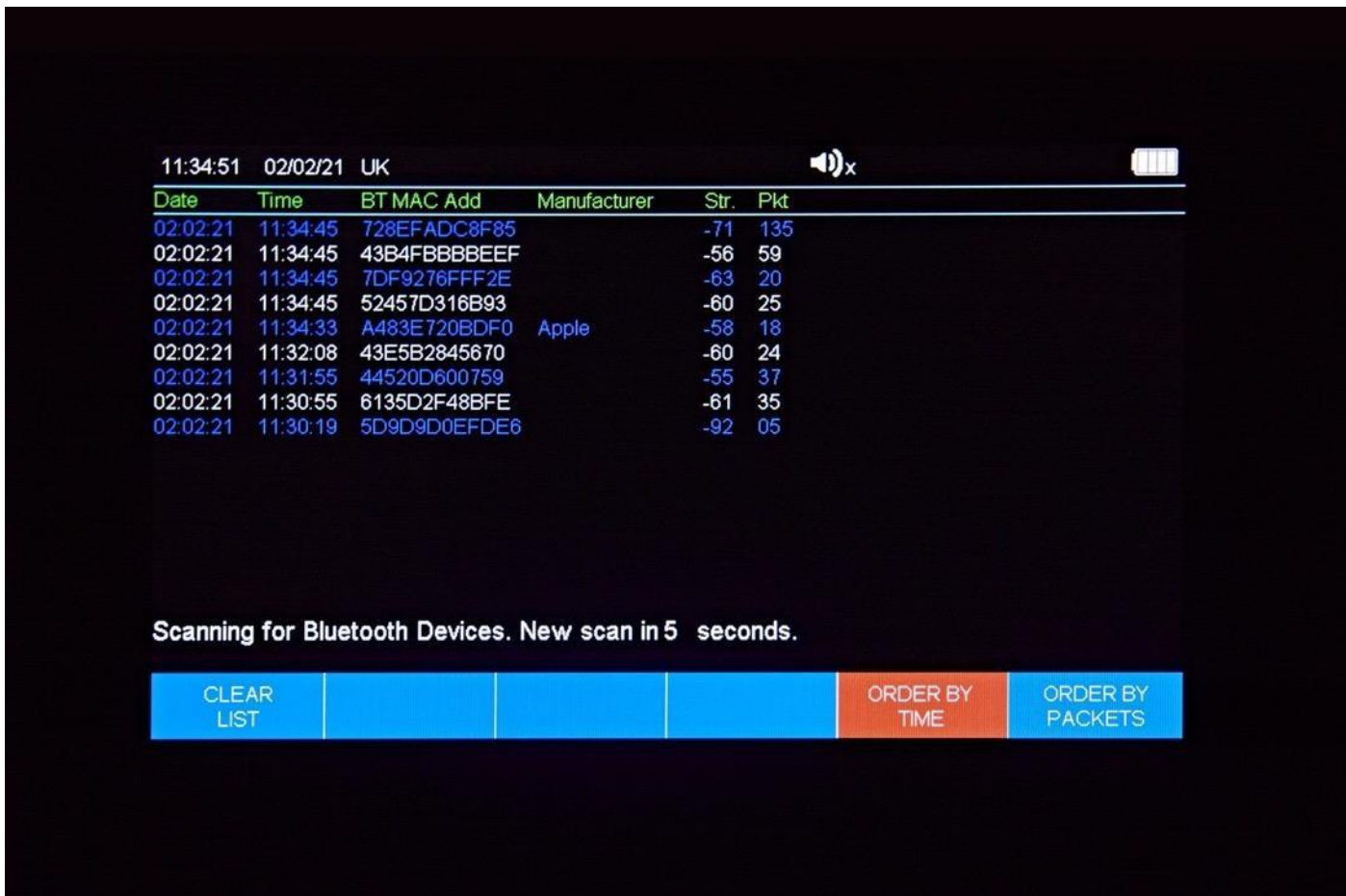
Bluetooth screen showing a list of detected Bluetooth devices
