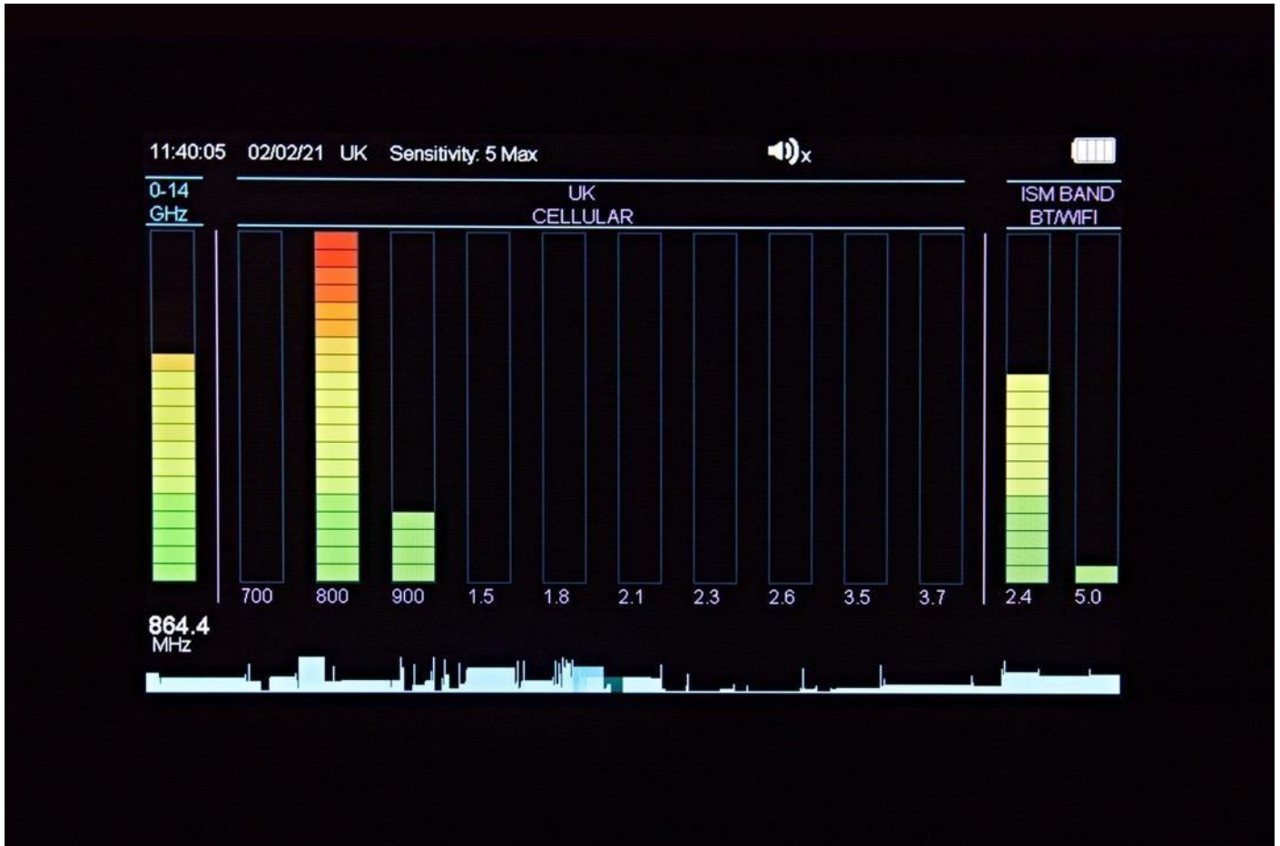
Main screen of the WAM-X25 showing live detected signals
